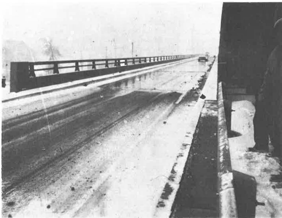
Figure 10. Heated ramp during heavy snow storm in winter of 1963-1964 showing experimental area, Phase II (off-ramp) complete melting of snow in heated area; filled approach road, where no heating elements installed, kept free of ice due to heat dragged by tires from heated area.
