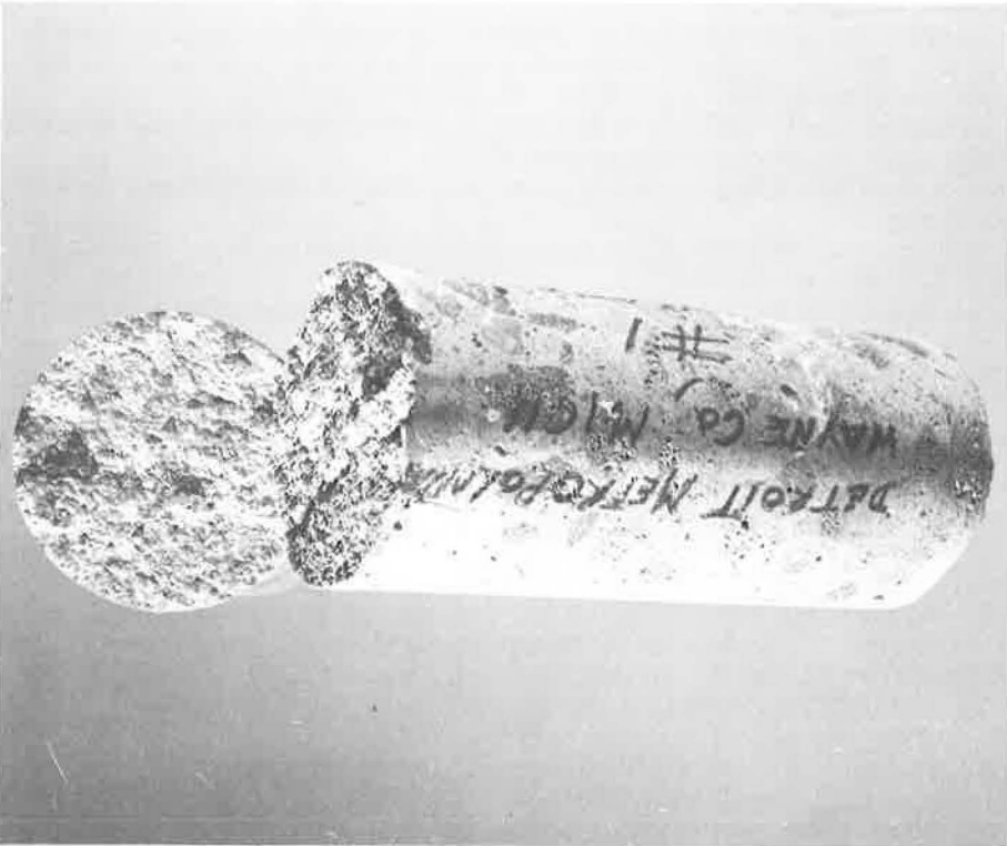
Figure 3. Core showing break in base pavement at Detroit.
