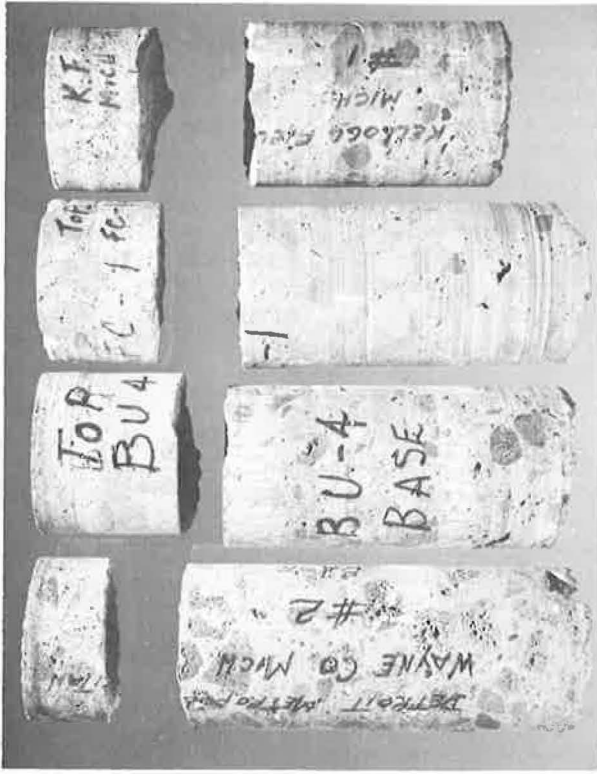
Figure 4. Cores showing breaks in base pavements at (l. to r.) Detroit Metropolitan Airport; Bunker Hill Air Force Base, Ind.; Fort Campbell, Ky.; and Kellogg Field, Mich.
