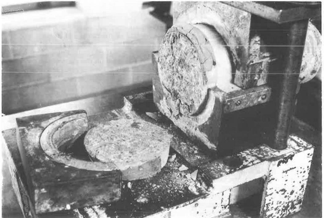
Figure 2. Laboratory jig for shearing cores.
