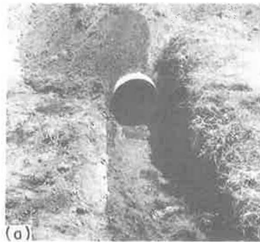
Figure 13. Field test site, IV-SCr-5-A, right of Sta. 530±: (a) aluminum invert sample approximately 0.8 yr of test; (b) cross-section of aluminum, nonperforated section.
