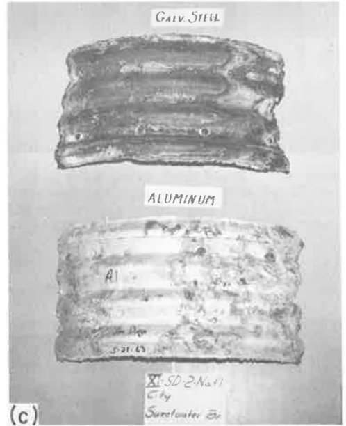
Figure 18. Field test site, XI-SD-2-Nat.Cty at Sweetwater Creek: (a) field test site at high tide; (b) sample removed from culvert inverts after approximately 1.6 yr of test; (c) backfill side of same culvert samples.
