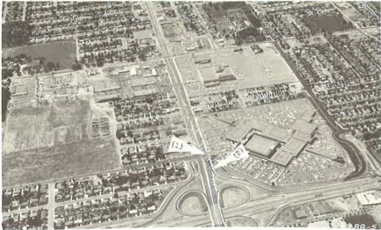
Figure 6. Example of inadequate access control on a crossroad beyond end of ramp.
