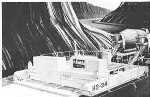
Figure 16. Drawing of HS-24 slip-form paver used in California.
