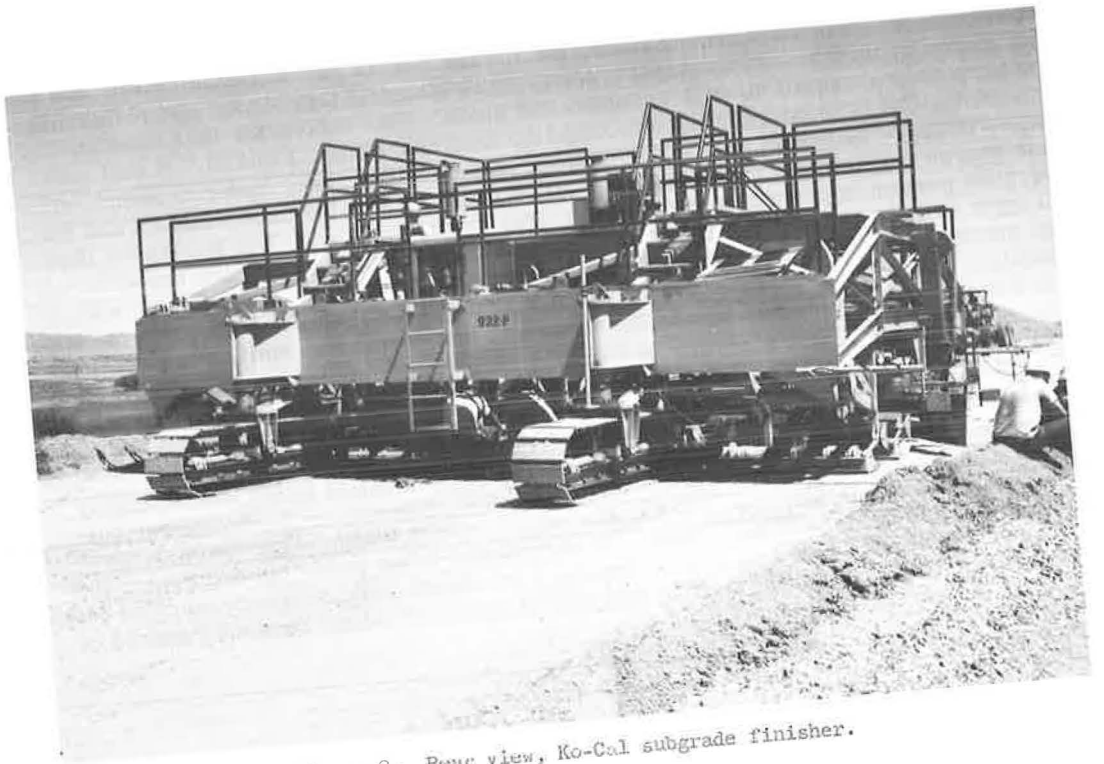
Figure 1. Front view, Ko-Cal subgrade finisher.
