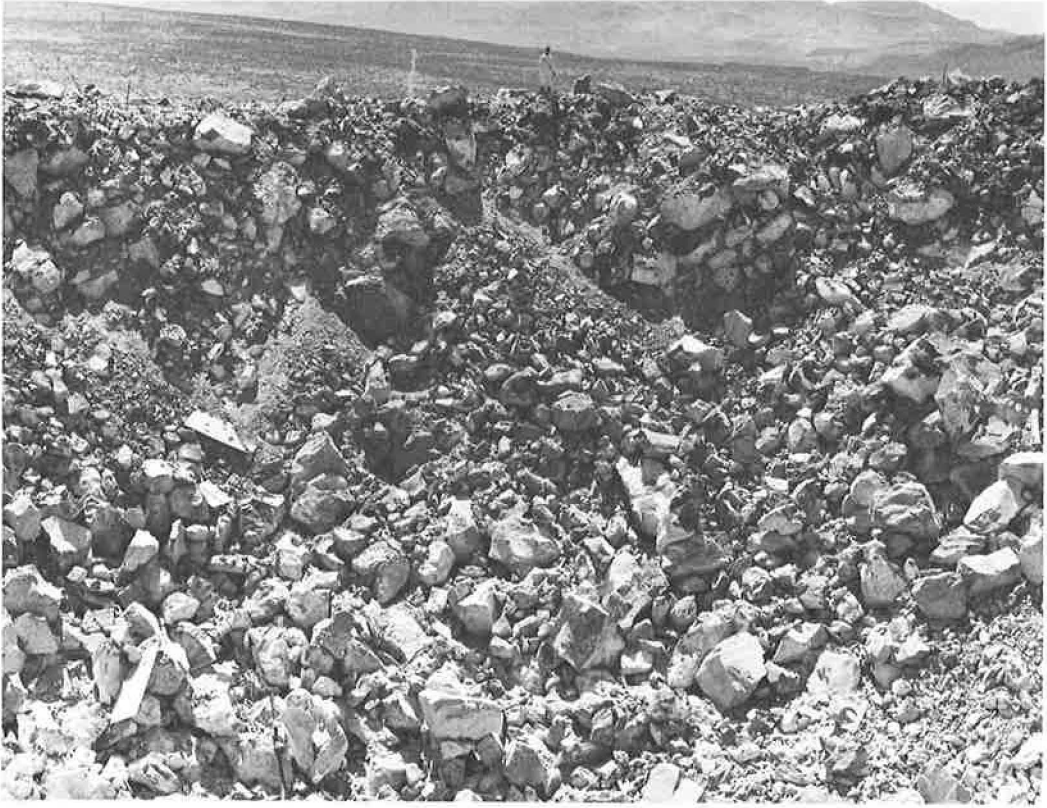
Figure 6. View across Danny Boy crater showing general nature of explosion-broken rock (note man standing at upper center of photograph).
