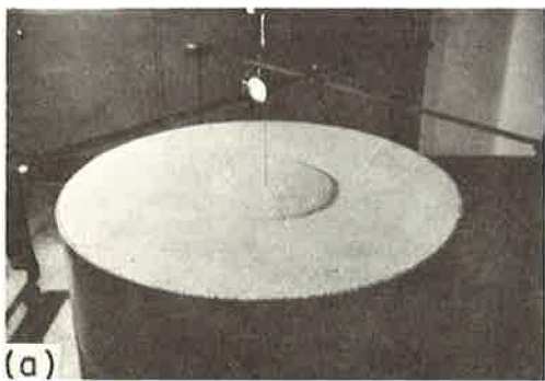
Figure 5. (a) failure circle developed by shallow anchor ( h/d < 6 ); and (b) shape of two-dimensional failure surface developed by 3-in. wide anchor.
