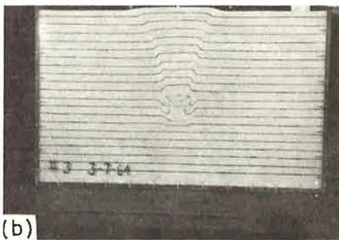
Figure 5. (a) failure circle developed by shallow anchor ( h/d < 6 ); and (b) shape of two-dimensional failure surface developed by 3-in. wide anchor.
