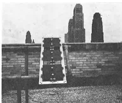
Figure 6. Carbon steel and high-strength low-alloy steel specimens on roof, Chicago, Ill.
