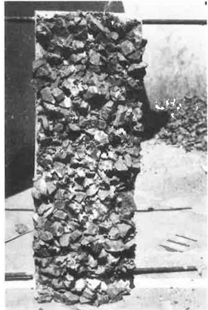
Figure 21. Underside of 3-ft by 1-ft by 6-in. slab bonded to water-bound macadam base (dry) after test.
