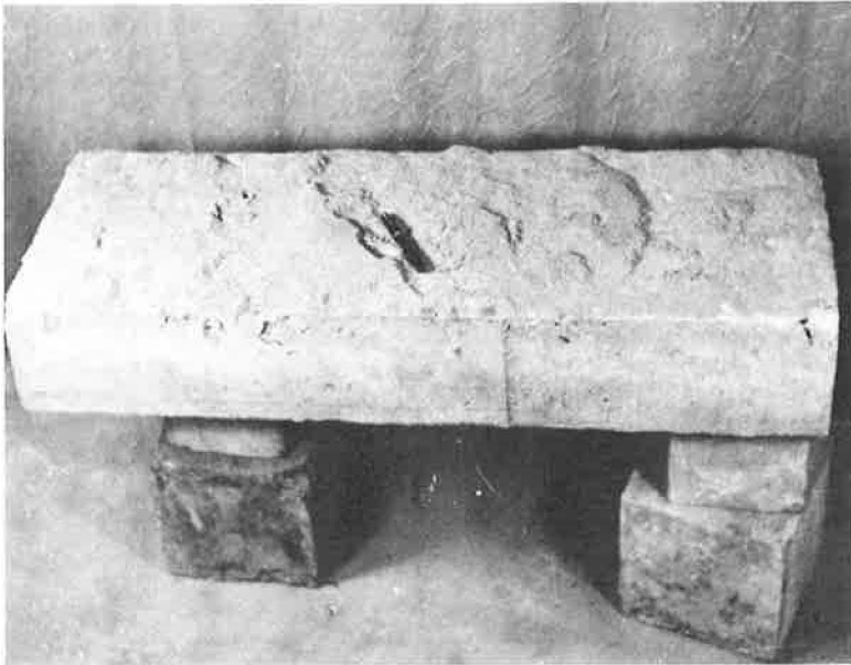
Figure 17. Underside of 3-ft by 1-ft by 6-in. slab bonded to a dense sand base, with masses of sand sticking to surface.
