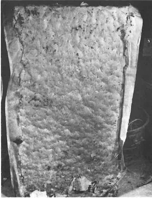
Figure 8. Underside of 4-ft by 2-ft by 6-in. slab on insulation paper over water-bound macadam base, showing scratches on paper due to pushing of slab.
