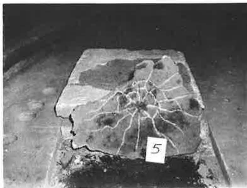
Figure 20. Bottom surface of typical cones punched out of pavement in static load tests.
