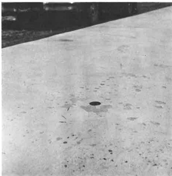
Figure 30. Blisters formed on exposed surface of experimental slab from dried exudation product.
