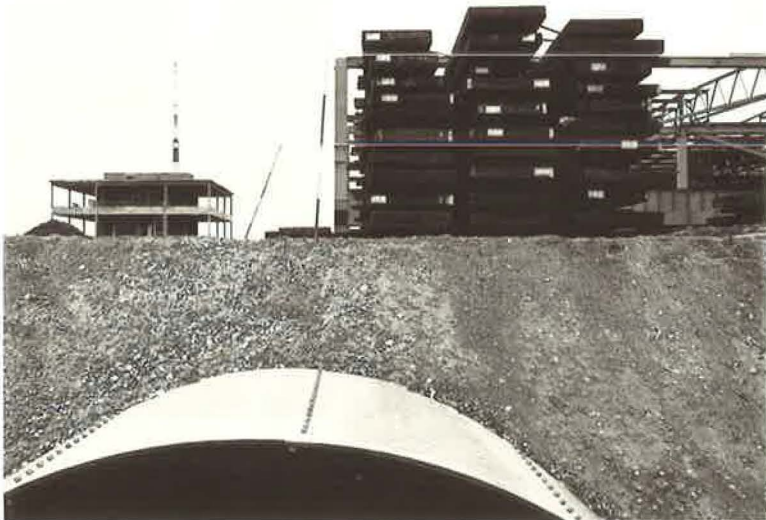
Figure 12. Test structure under load of 151.32 tons applied in 6.89-ft off-center position.
