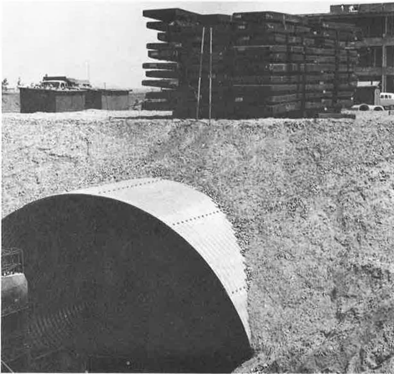
Figure 8. Live-load test, test structure with 151.32-ton axial load.
