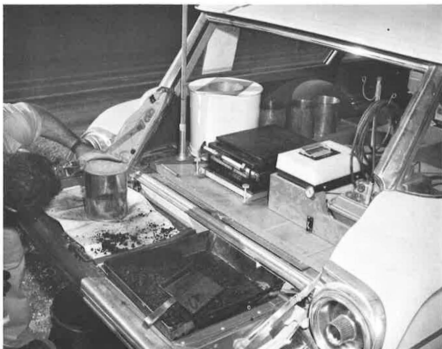
Figure 9. Fitting transite lid to container.
