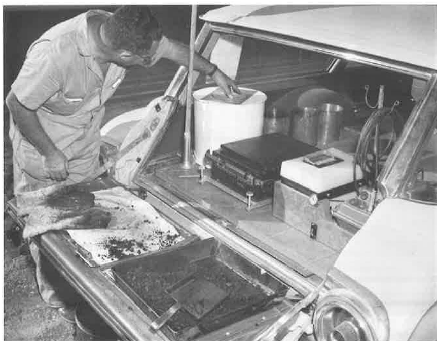
Figure 11. Replacing transite lid on container.
