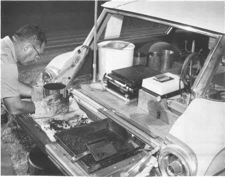
Figure 7. Settling material with rotating motion.
