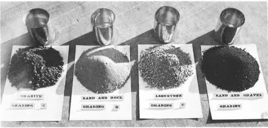
Figure 1. Aggregate materials for master standards.
