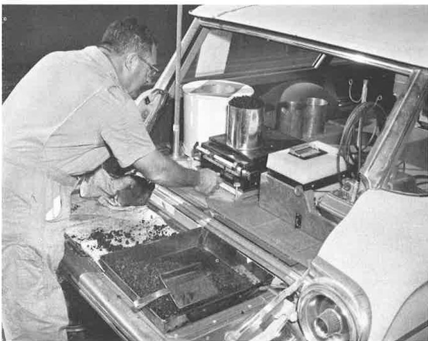
Figure 6. Weighing asphalt sample.
