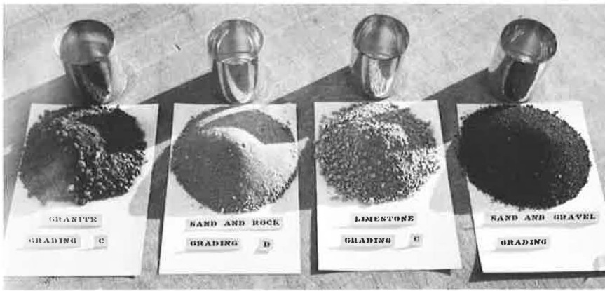
Figure 1. Aggregate materials for master standards.
