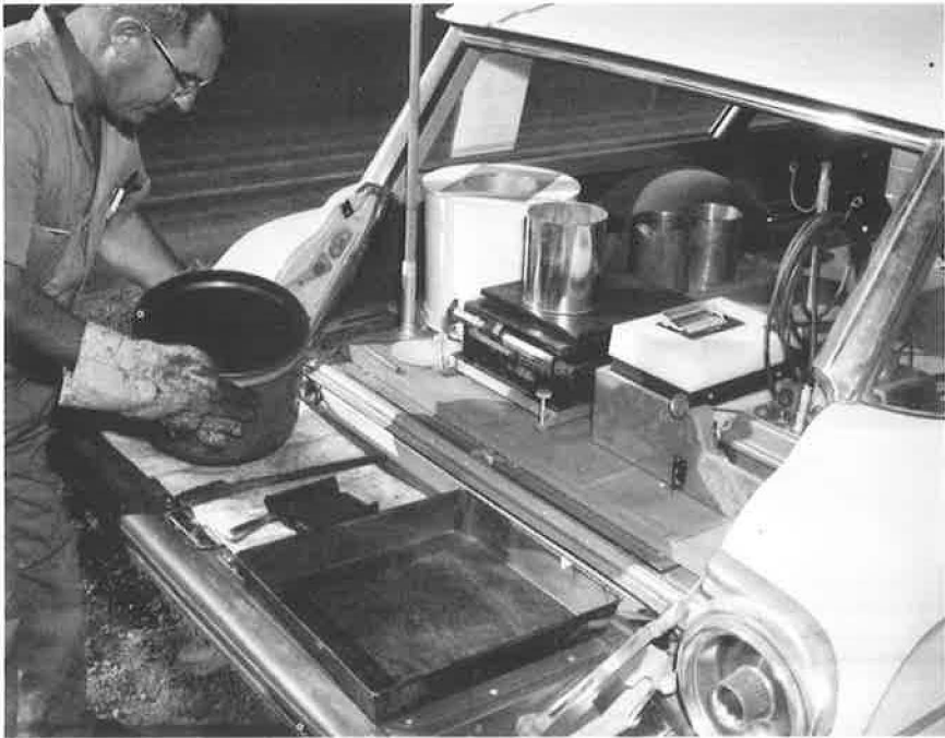
Figure 3. Asphalt sample from the roadway.
