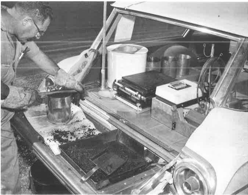
Figure 8. Leveling the material.
