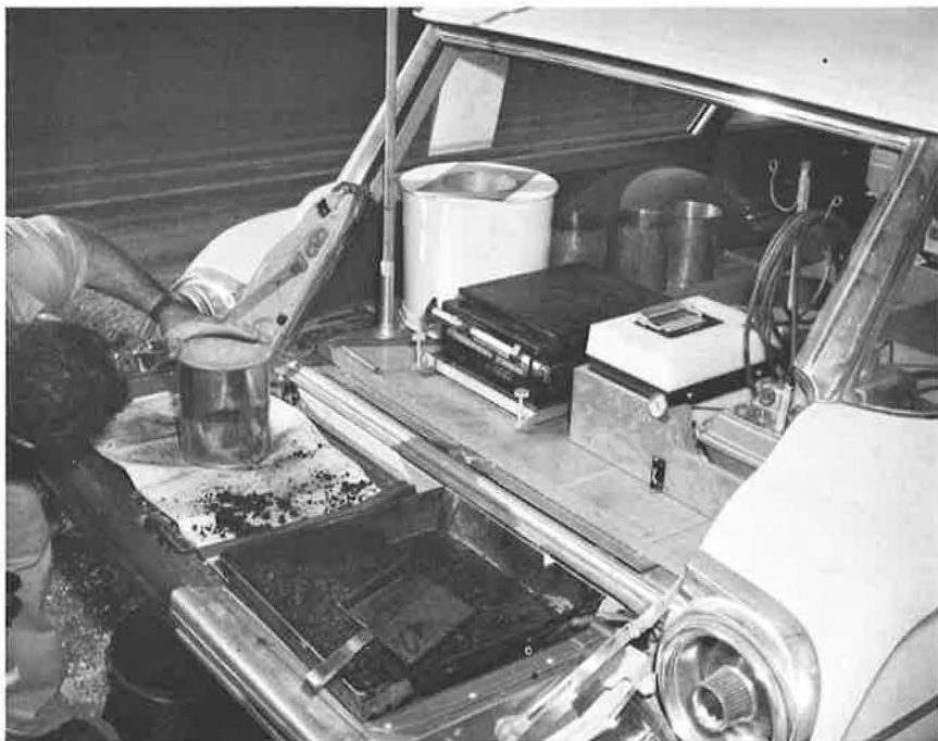
Figure 9. Fitting transite lid to container.
