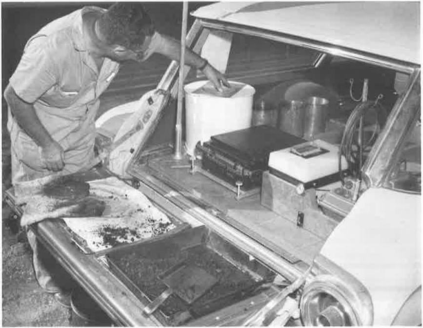
Figure 11. Replacing transite lid on container.
