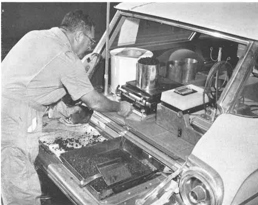
Figure 6. Weighing asphalt sample.
