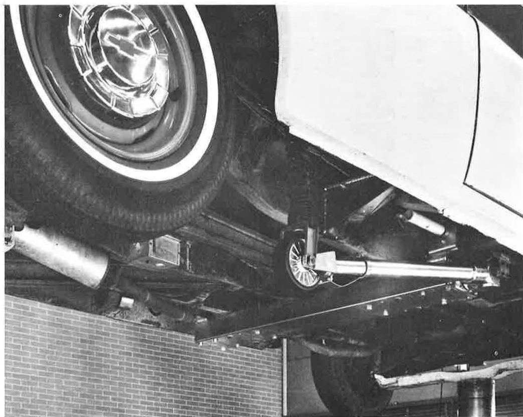
Figure 13. Road wheel assembly mounted on truck.
