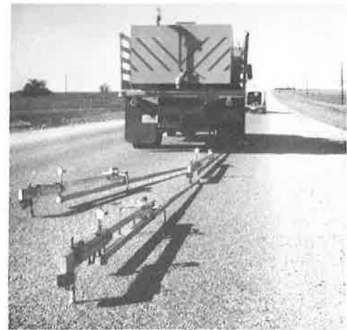
Figure 11. Three Benkelman beams sometimes used in 1964 correlation study: beam in background measured deflection at wheel load; two beams in foreground registered movement at the supports of distant beam.
