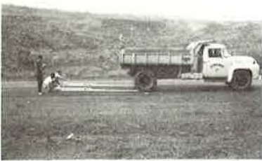
Deflection measurement using the Benkelman beam—CGRA method, initial position.
