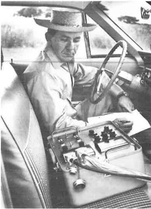
Figure 7. Dynaflect is controlled and deflections recorded inside towing vehicle.
