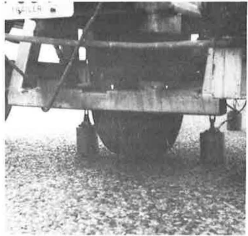
Figure 9. 1964 model in which force was transmitted to roadway through a single steel wheel.
