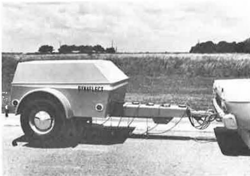
Figure 1. Dynaflect halted for measuring roadway deflections; force generator is located in covered trailer; deflection pickups rest on pavement beneath trailer tongue.
