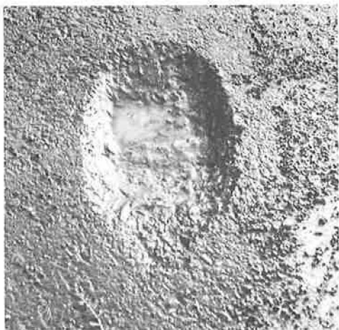
Figure 9. Test no. 17 (chain on new asphaltic-concrete shoulder): maximum depth of scour 1.5 in.
