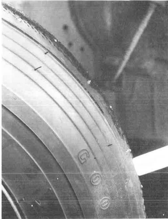
Figure 21. Wear on front tires after 21 series of stops and starts (400 mi total travel).
