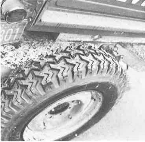
Figure 1. New OK Rubber Co. "extra traction" tread with 72 tungsten carbide studs.
