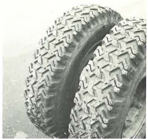
Figure 16. Initial studded tires after removal at 2,940 trips (27 hr): rear tire, left; front tire, right.
