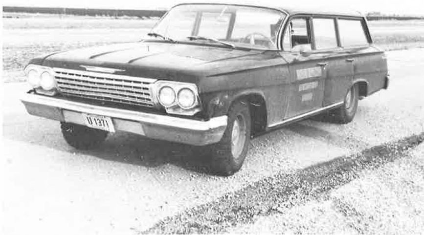
Figure 4. Chevrolet station wagon with studded tires on all four wheels.
