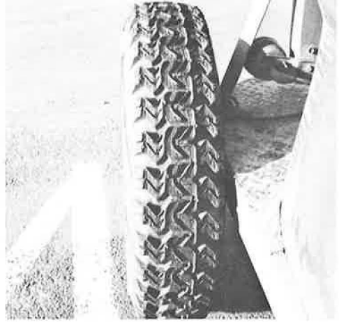
Figure 2. Tire similar to Figure 1, after 21st test spin; tread 50 percent gone; one stud lost.
