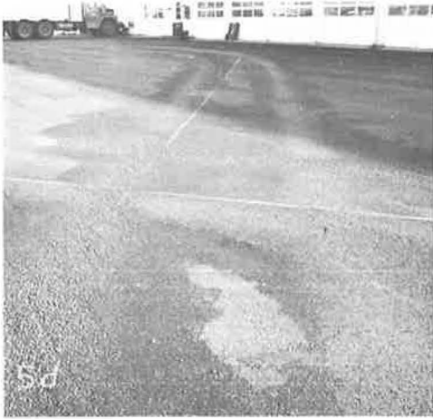
Figure 27. Cross-over area at 46 hr (5,330 trips).
