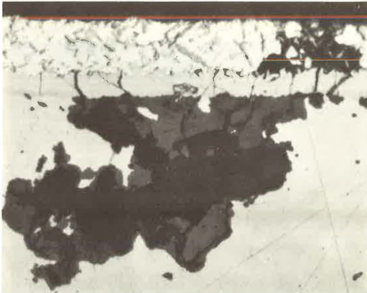
Figure 17. Rusting of base steel under intact aluminum coating at pitted area of Figures 12 and 13—some of the fractures in the aluminum-iron alloy layer of coating have become channels for oxidation process (section 625 X, after 25% reduction in reproduction; unetched after high pressure lapping on paper over plate glass).
