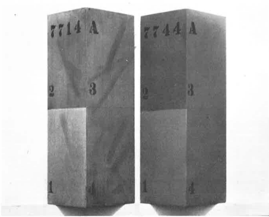
Figure 2. Comparison of control New York State system (left) and experimental basic lead silico chromate system (right) after 19 months exposure at 45° South on Long Island.
