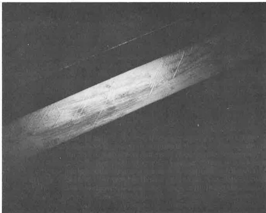
Figure 4. A demonstration of irregular gloss experienced with gray-green finish coat paint.
