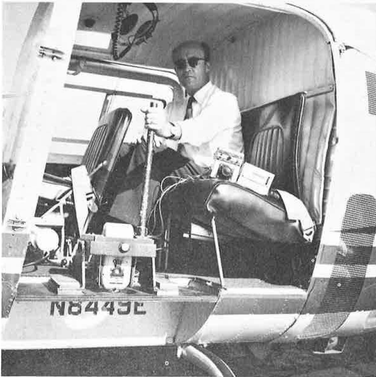
Figure 3. Camera and auxiliary equipment installed in helicopter.
