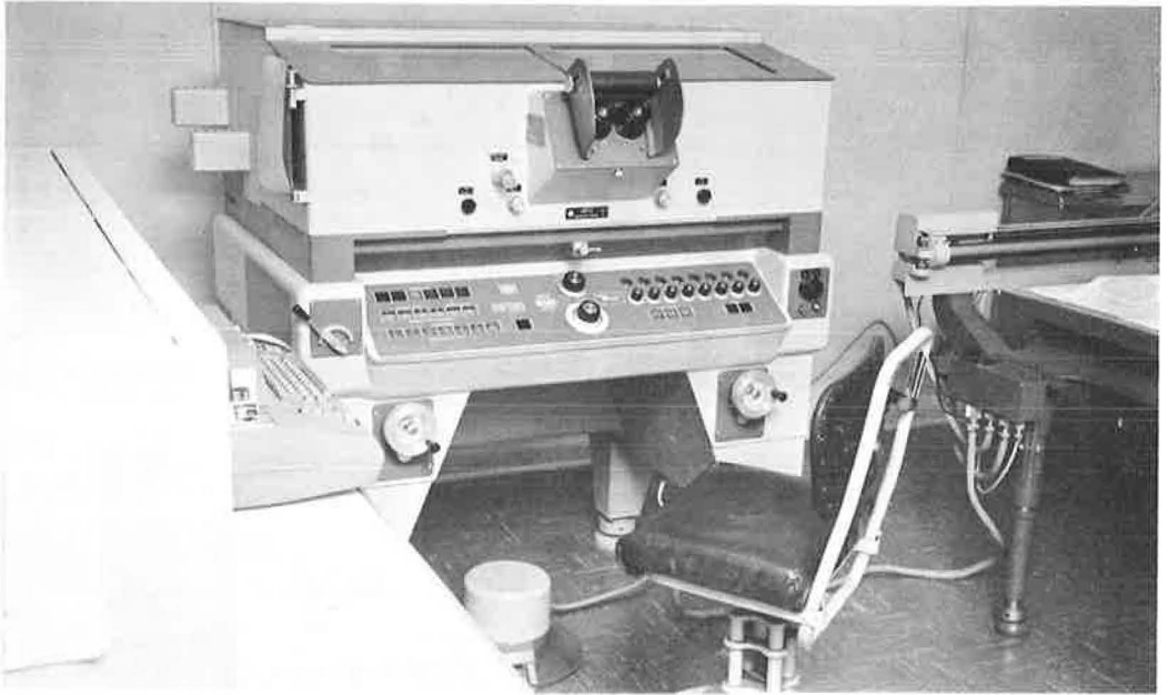
Figure 5. Nistri Analytical (Stereoscopic) Plotter, Model AP/C.
