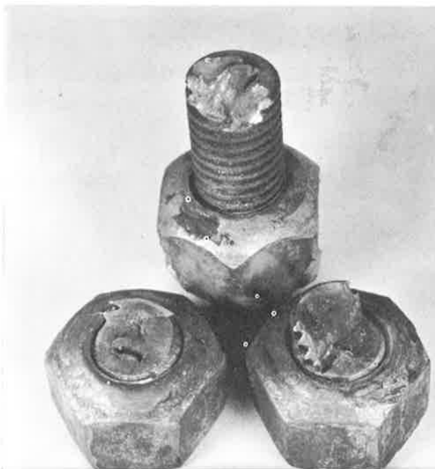
Figure 4. Broken bolts obtained from Wolf Creek.
