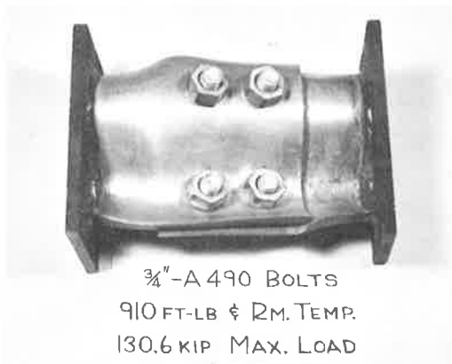
Figure 9. Typical plate failure.
