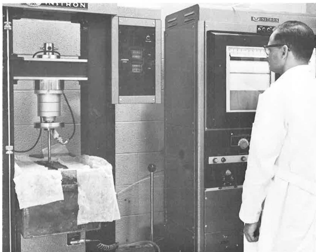
Figure 1. Penetration test in progress.
