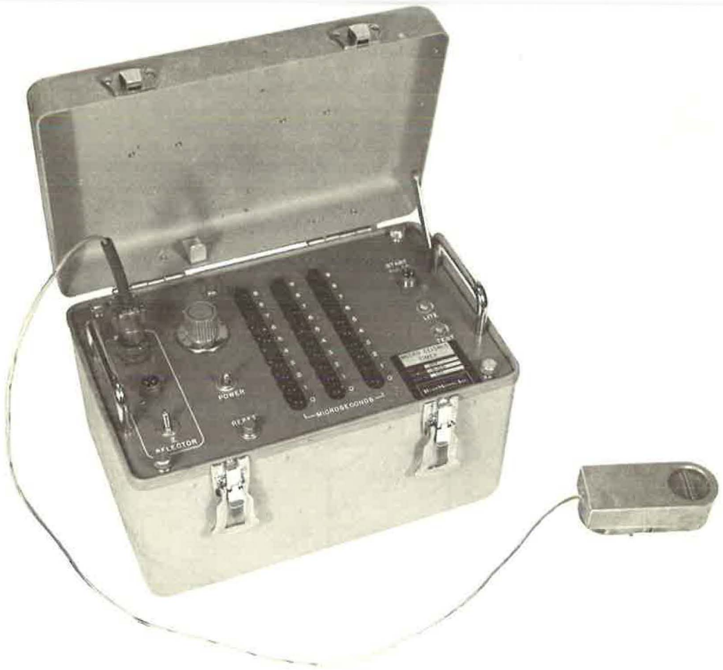
Figure 8. Microseismic timer and pickup.
