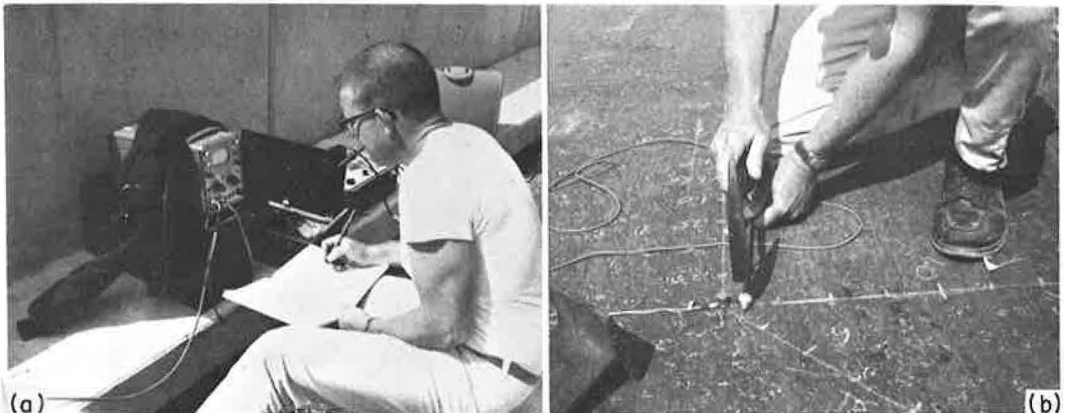
Figure 1. Evaluation of microseismic refraction method: (a) observing travel times on portable oscilloscope triggered by impacts; (b) refraction survey line, impact device and accelerometer.
