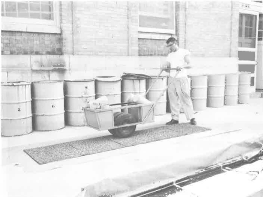
Figure 15. Pneumatic roller used to seat stone on laboratory surface treatments.
