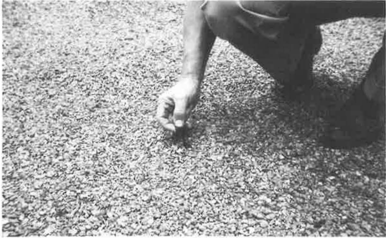
Figure 62. Adhesion of asphalt to type F material is very good.
