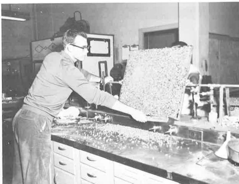
Figure 16. Completed surface is tilted 75 deg and brushed to remove loose stone.
