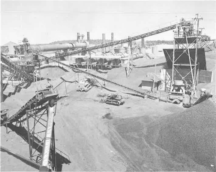
Figure 5. General view of commercial lightweight aggregate plant: crushing and sieving is in right foreground.
