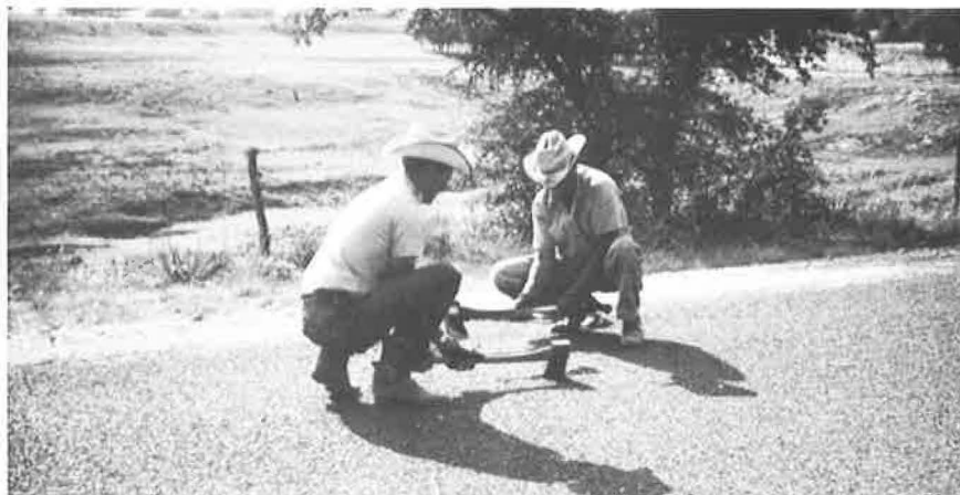
Figure 41. Cutting a field sample with an ax.
