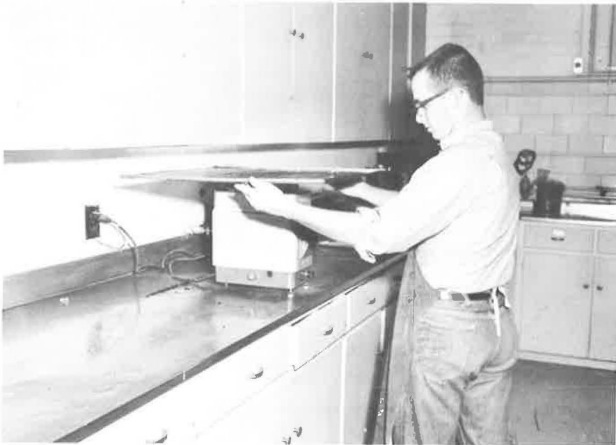
Figure 13. Asphalt coated board being weighed to measure application rate.
