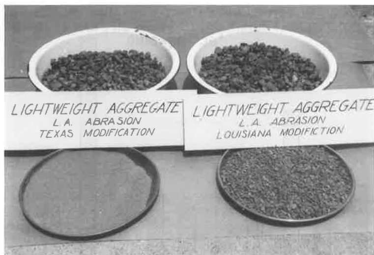
Figure 37. Type F materials after testing by Texas and Louisiana methods for Los Angeles abrasion.
