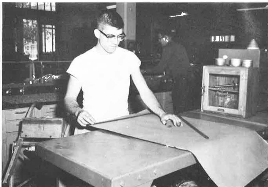
Figure 9. Laboratory surface treatment board being covered with paper.
