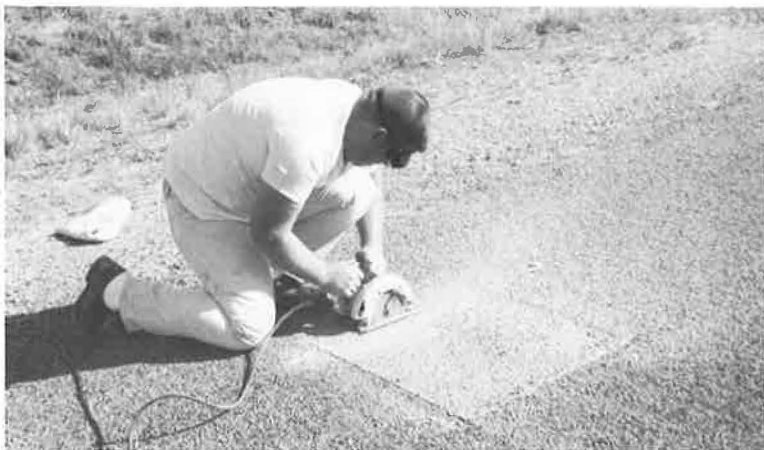
Figure 40. Cutting a field sample with a portable saw.
