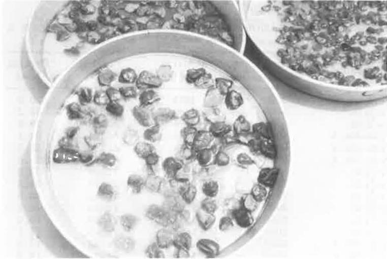
Figure 38. Type F material after freezing in water.
