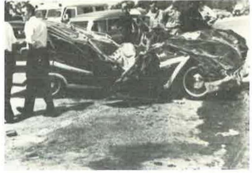
Figure 15. Roof-to-roof impact due to deep drainage ditch in center of median shown in Figure 14. Four killed.
