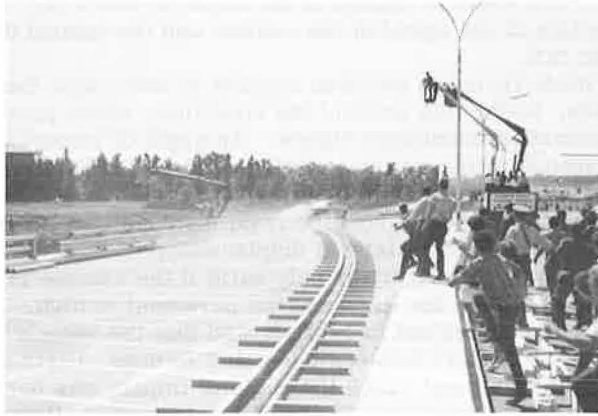
Figure 5. Projection system for the impacting vehicles for all the tests, except for two tests on guide rail Model H (just before impact).
