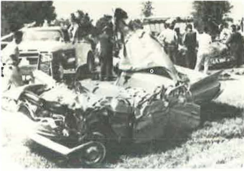
Figure 15. Roof-to-roof impact due to deep drainage ditch in center of median shown in Figure 14. Four killed.
