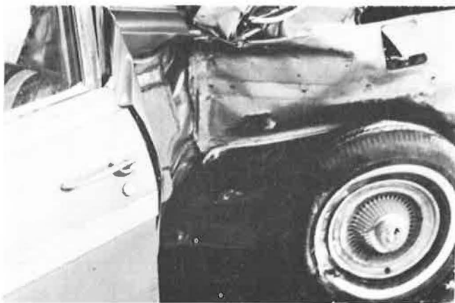
Figure 18. Vehicle "snagged" by guardrail, spinning it into bridge railing. Shown is the point of impact, left rear door. One killed.
