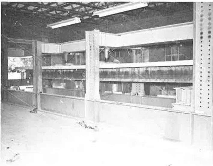
Figure 5. T-beam test setup.
