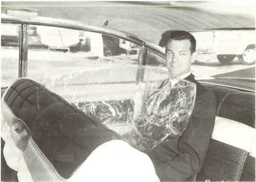
Figure 18. Mockup of an automobile airstop restraint, which should include airseat,
