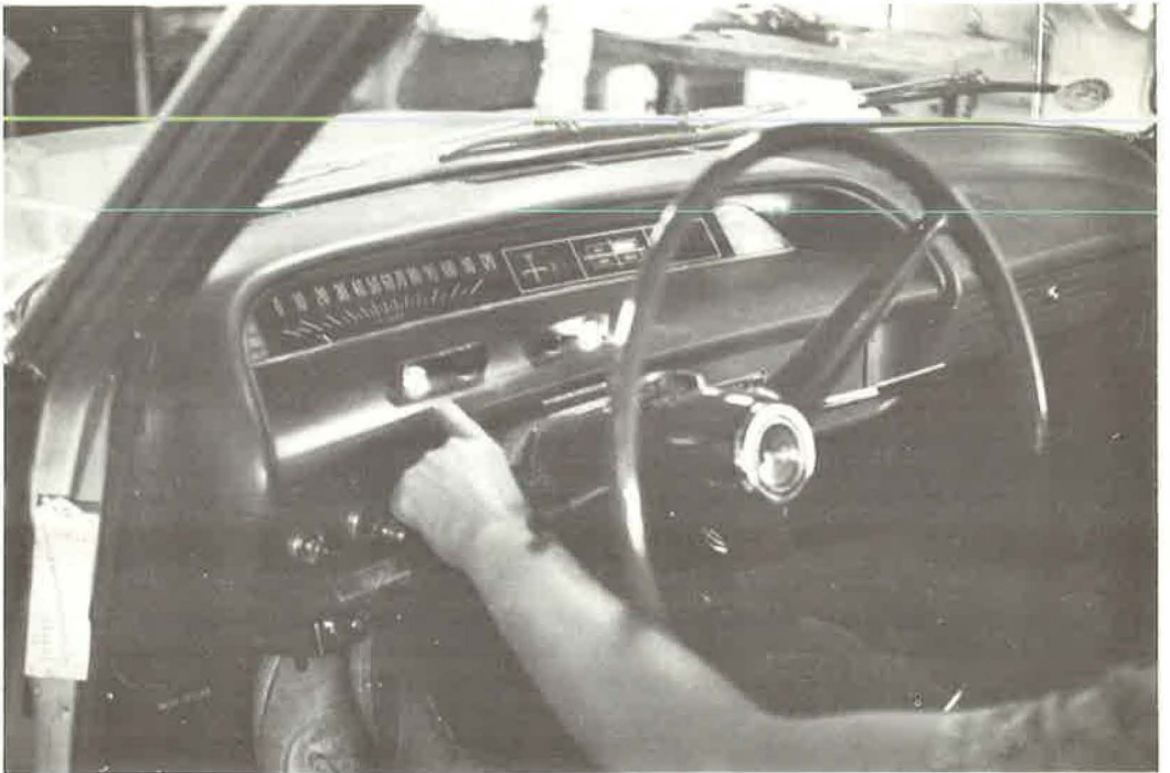
Figure 5. Display lights on dashboard of following car.
