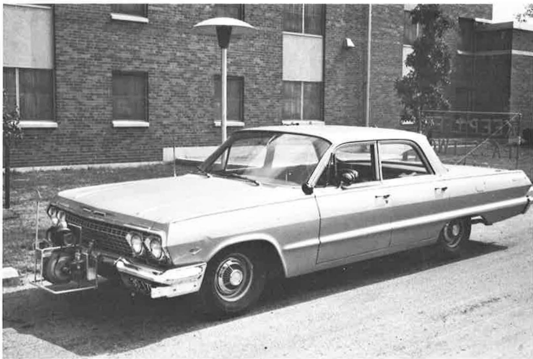
Figure 2. Following car with mechanical take-up reel.
