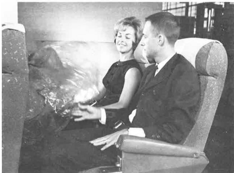
Figure 19. Automatic roll-up of the airstop chest airbag.
