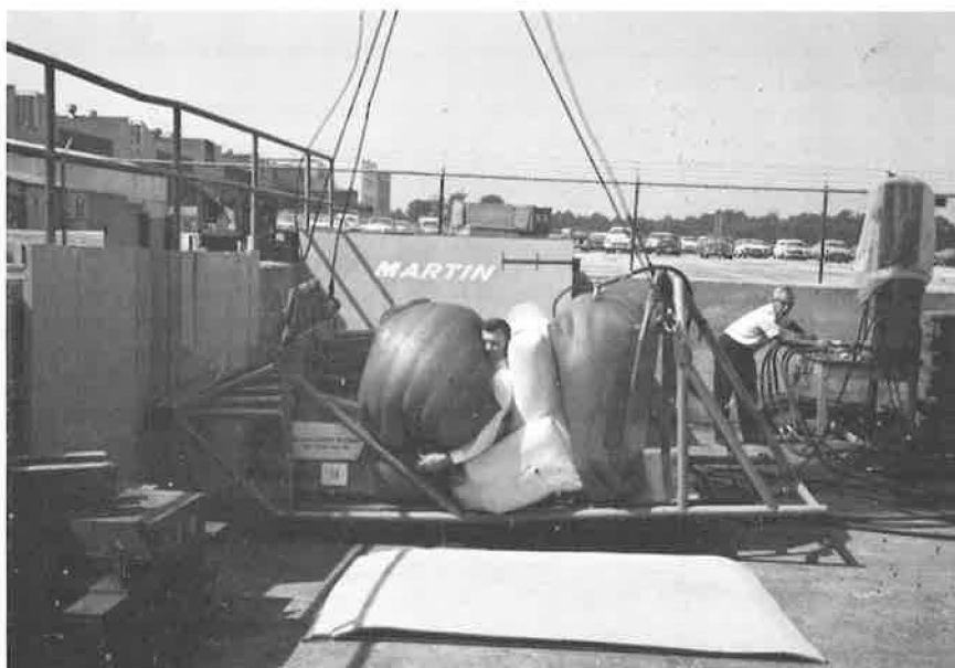
Figure 5. Swing impact of complete airstop system with airseat (impact velocity 16 ft/sec; human subject).
