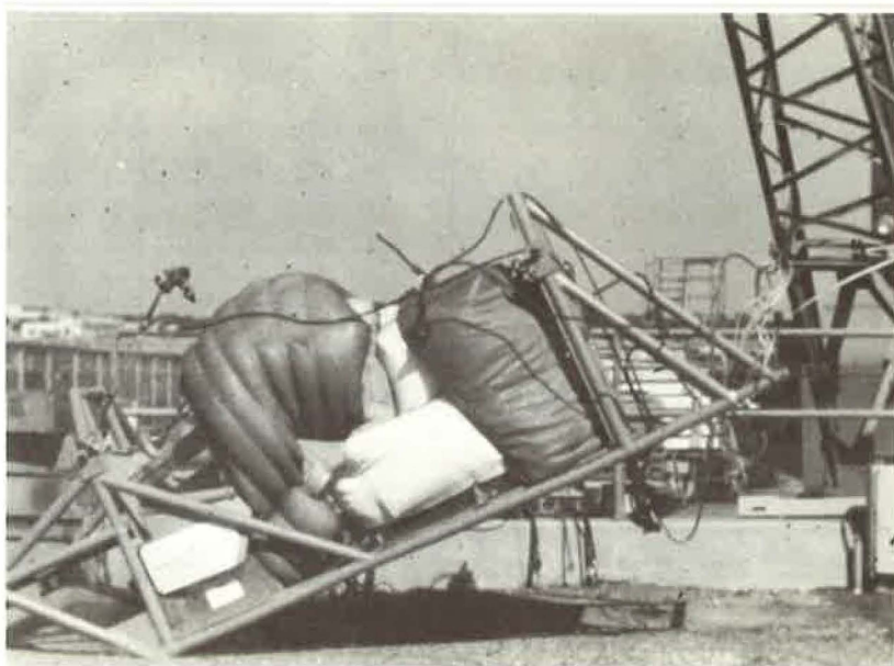
Figure 21. Crane drop of the complete system, during impact (impact velocity—32 ft/sec; dummy subject).
