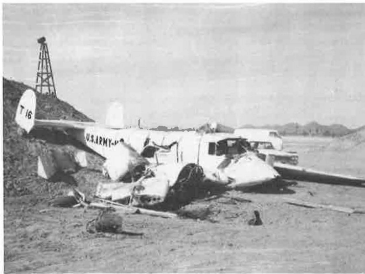
Figure 12. First C-45 after 100-mph crash (airseat is at torn fuselage position).
