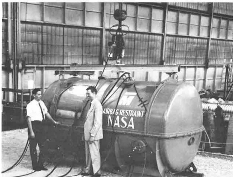
Figure 8. Test vehicle, pilot compartment airbag restraint system.
