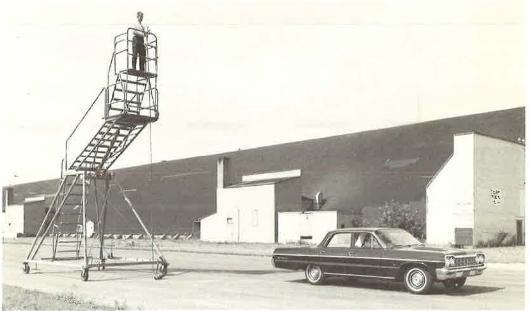
Figure 4. Apparatus used to create simulated rain condition.
