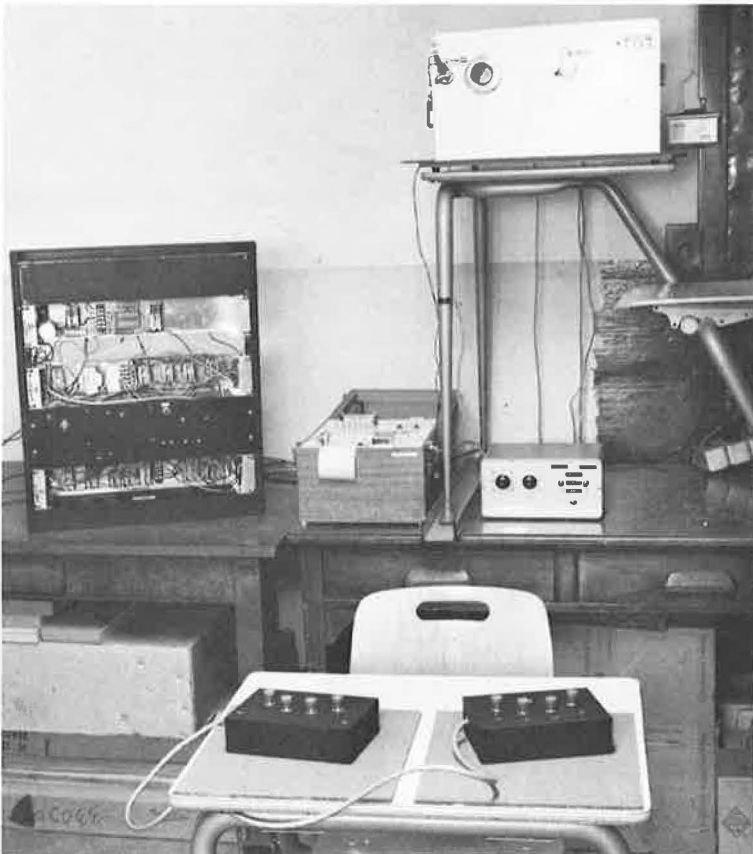
Figure 2. Response buttons, control, recording equipment and dual tachistoscope (upper right).
