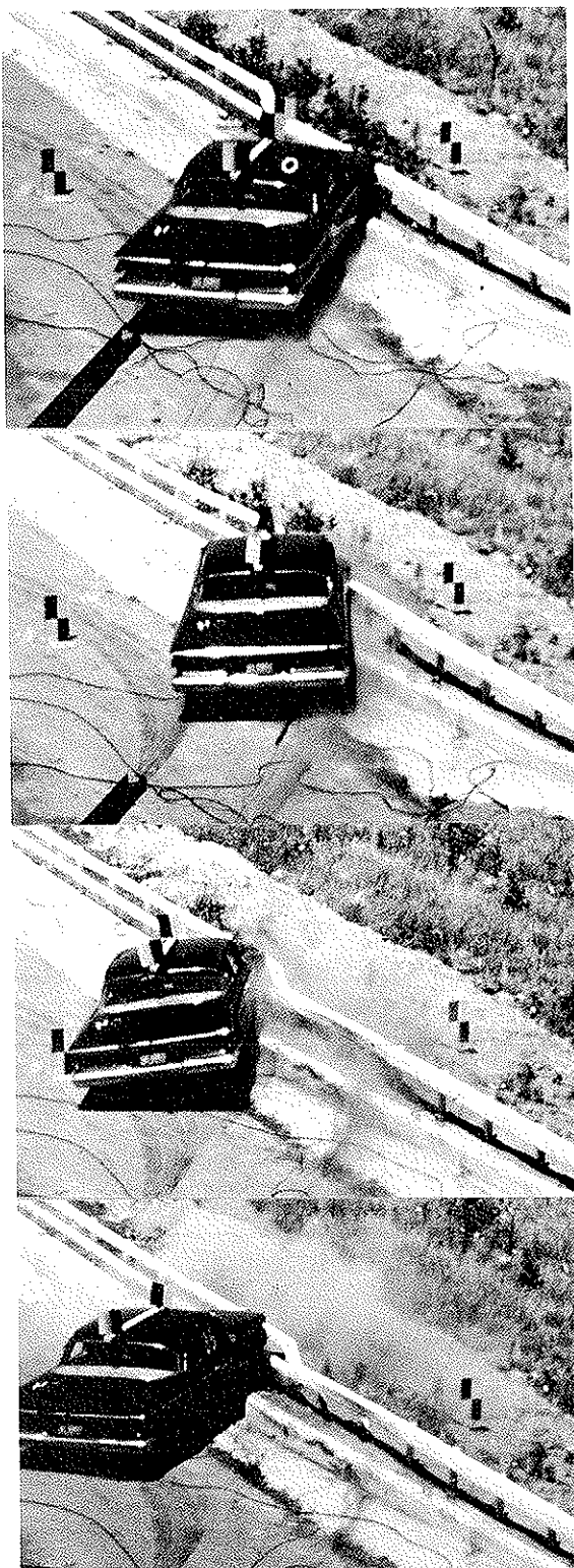
Figure 60. Box beam transition (Test 35).
