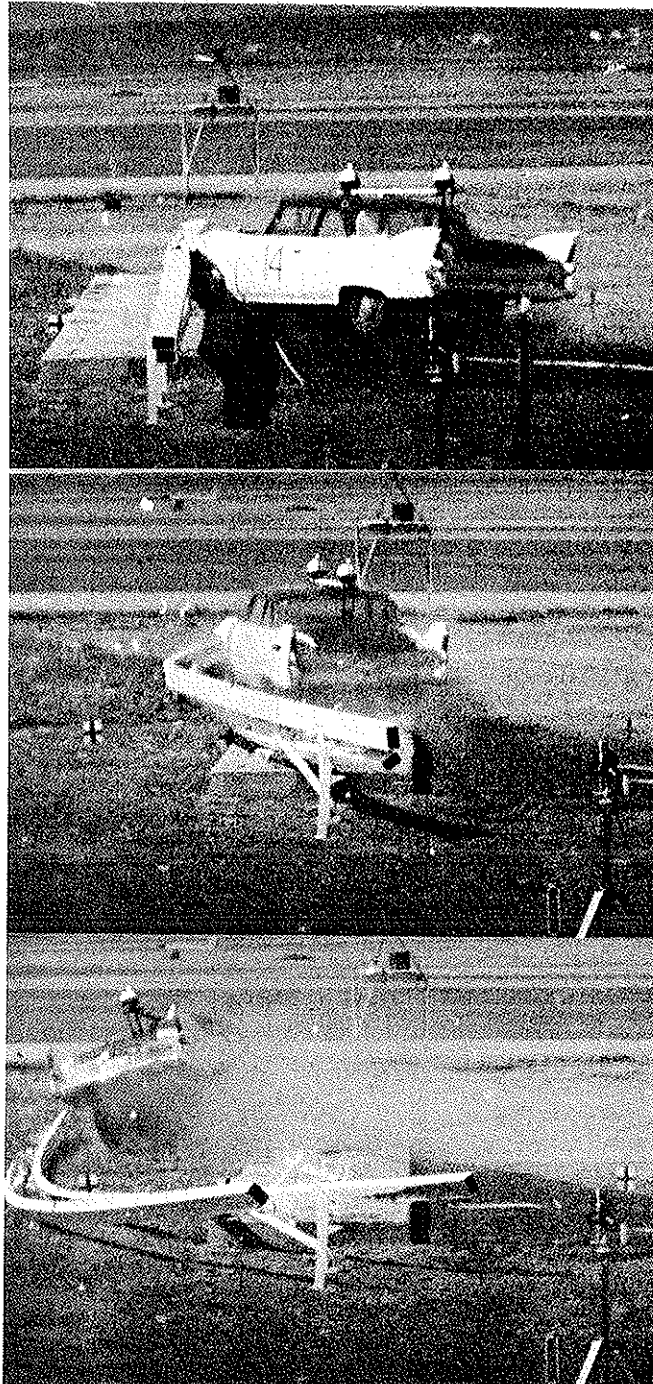
Figure 29. Box beam bridge rail (Test 14).
