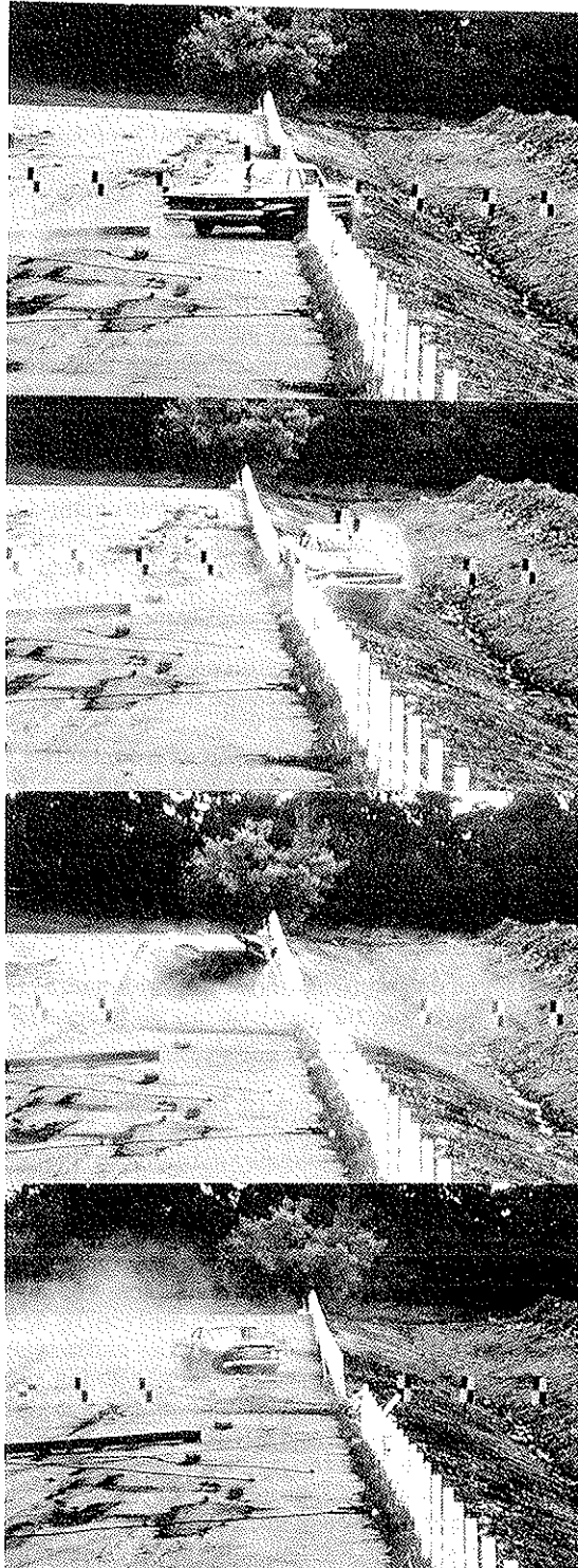
Figure 64. Cable guide rail (Test 20).
