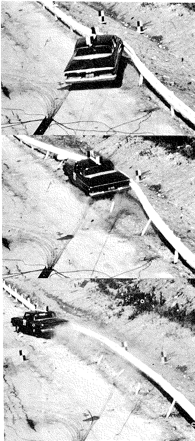
Figure 78. W-section guide rail (Test 39).
