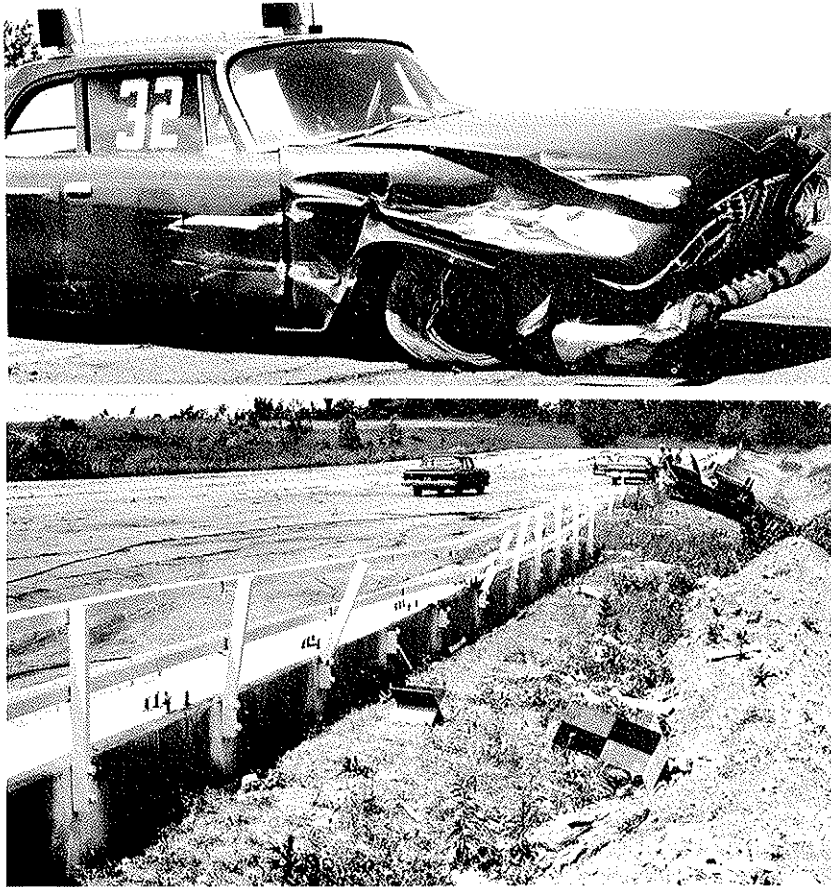
Figure 35. Car and rail after Test 32.
