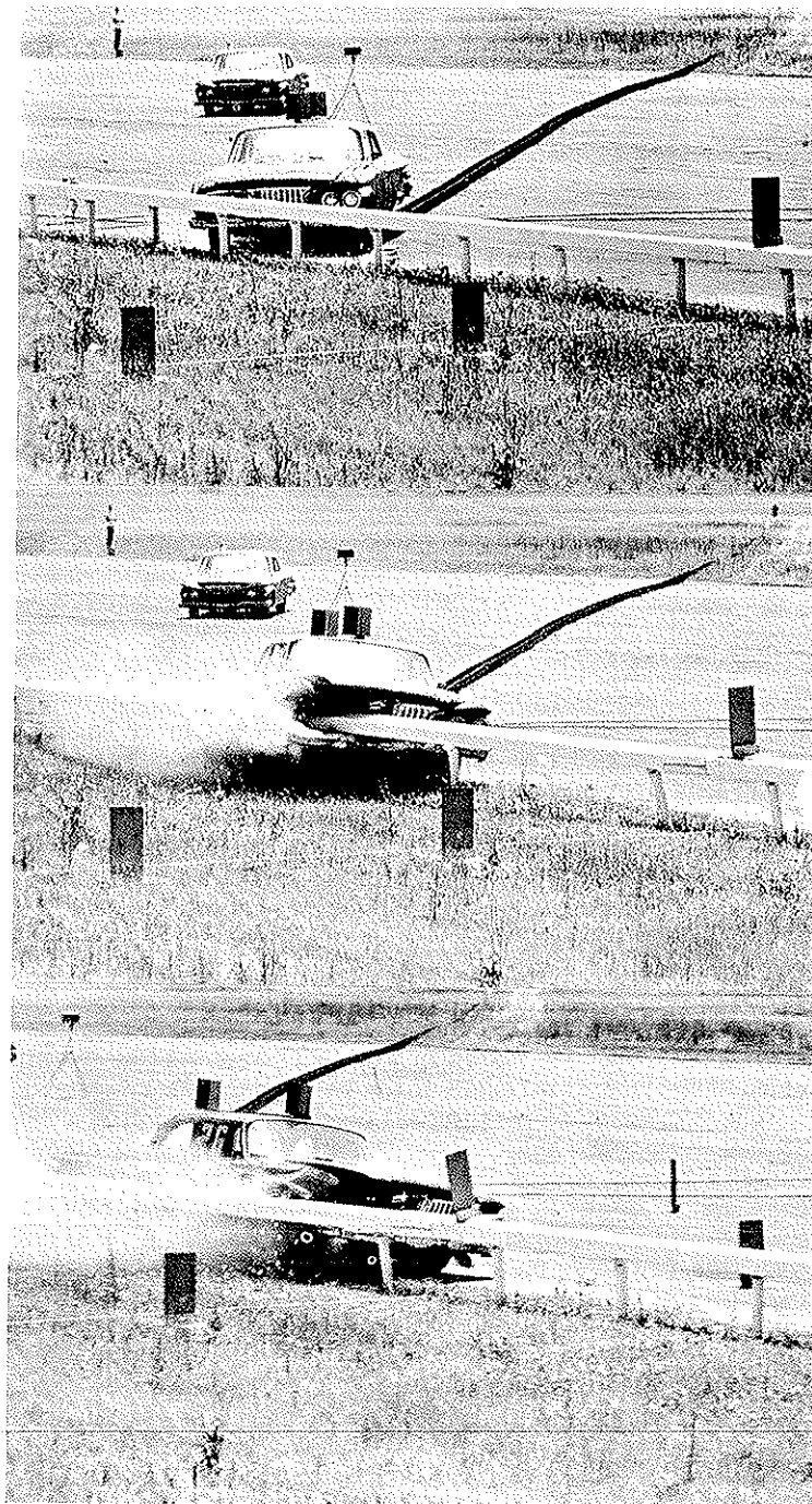
Figure 18. Box beam median barrier (Test 26).
