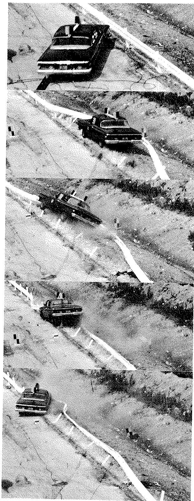
Figure 77. W-section guide rail (Test 38).
