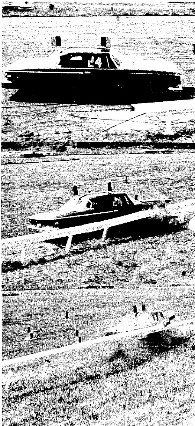
Figure 16. Box beam median barrier (Test 24).
