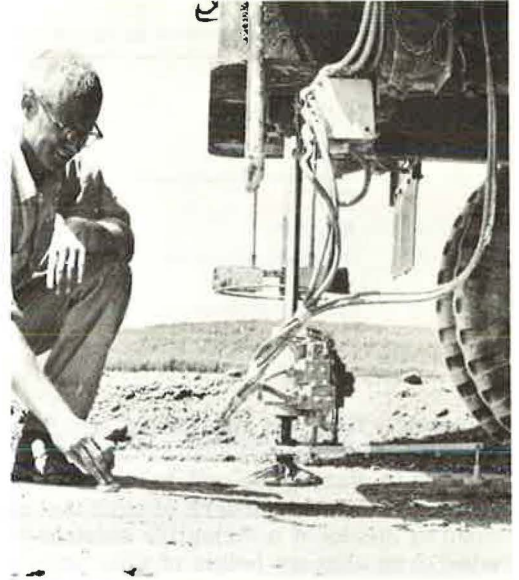
Figure 3. Bearing plate apparatus.
