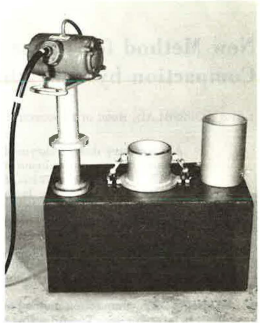
Figure 2. Vibrating tamper, test mold and collar.
