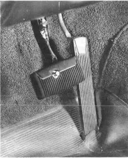
Figure 5. Push-button switch mounted in brake pedal.
