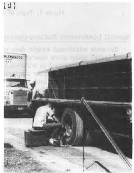
Figure 2. Loadometer station in operation: (a) loadometer flush with ground; (b) truck being guided onto loadometer; (c) wheel resting on loadometer; (d) loadometer being balanced and static weight read.
