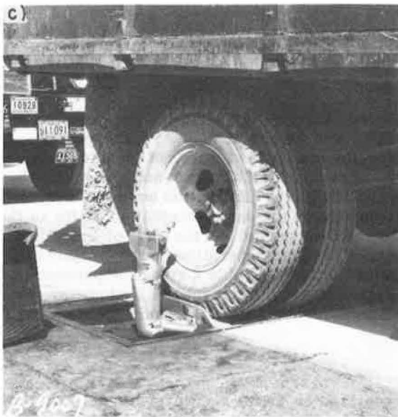
Figure 2. Loadometer station in operation: (a) loadometer flush with ground; (b) truck being guided onto loadometer; (c) wheel resting on loadometer; (d) loadometer being balanced and static weight read.
