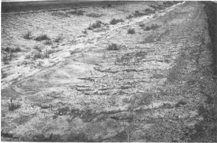
Figure 1. Salt accumulation in the soil of this median section of I-80 prevented the establishment of turf from seedlings during fall 1964 and spring 1965.
