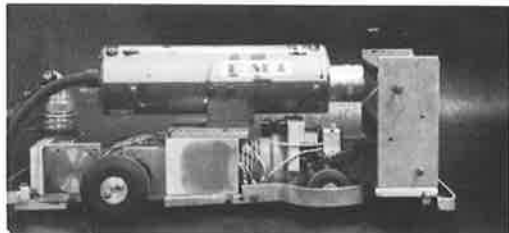
Figure 5a. Servo-controlled model vehicle with vidicon and periscope.
