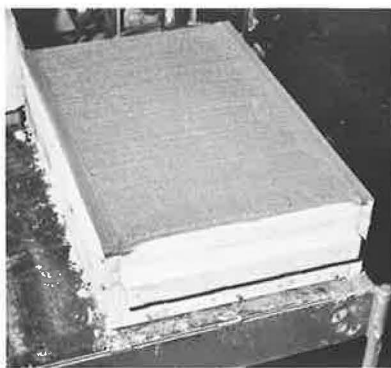
Figure 6. Finished block showing broomed surface.
