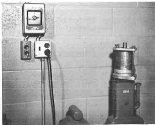
Figure 16. Abrasion test in progress.
