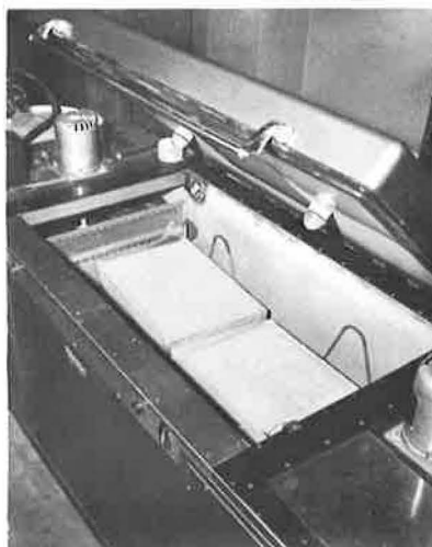
Figure 8. Blocks being frozen during early curing period.
