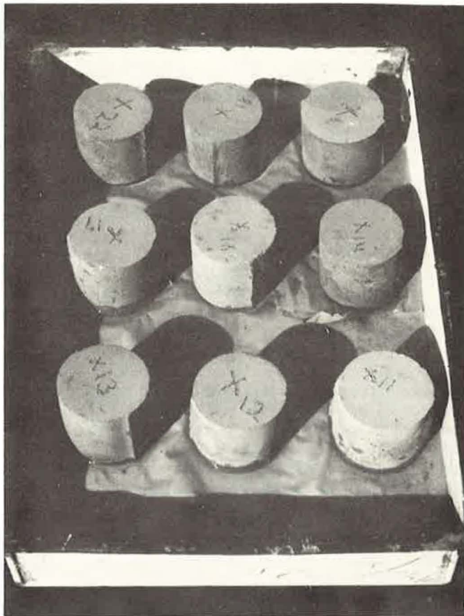
Figure 1. Specimen blocks in wetting tray.
