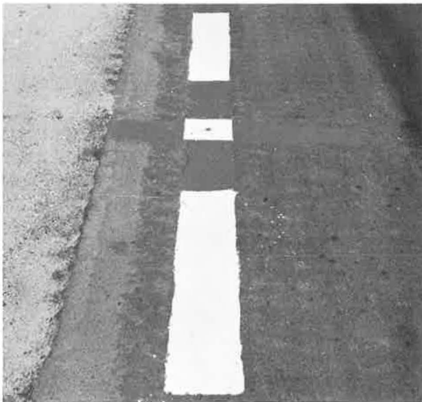
Figure 6. Premark target painted on shoulder of highway.
