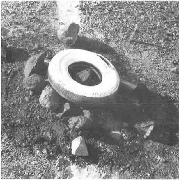
Figure 7. Premark of rock-mound section corner.
