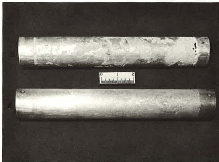
Figure 9. Aluminum specimens after exposure and removal of corrosion products: specimen A—exposure time, 16 months at site A; specimen B—exposure time, 32 months at site B.
