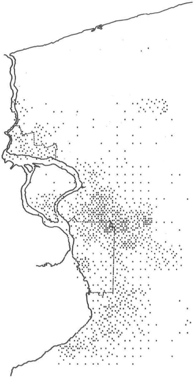
Figure 3. Trip-potential surface, 1962 (each dot equals 150 trips).
