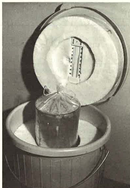
Figure 3. Complete autogenous curing container receiving test cylinder.
