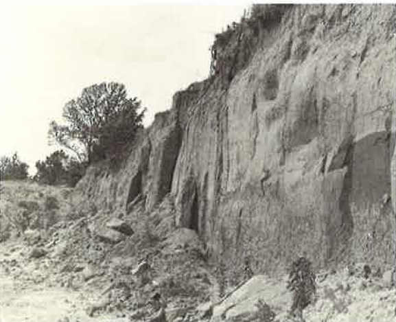
Figure 4. An example of "columnar slabbing" in loess in a gravel pit in Lauderdale County.
