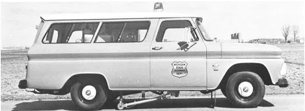
Figure 1. Michigan's GMR-type rapid travel profilometer.
