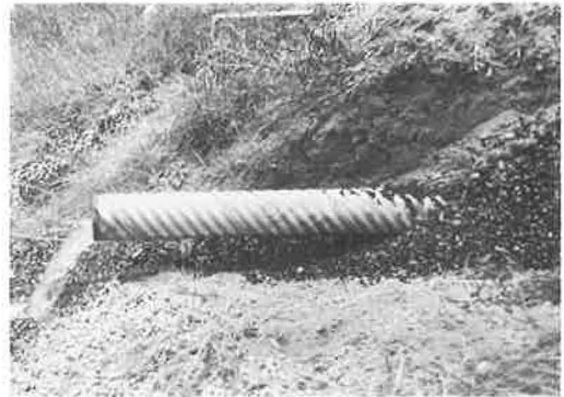
Figure 8. Flow from cross drain 2 to 3 minutes after sprinkling open-graded mix with watering truck.
