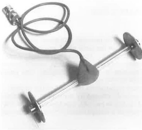
Figure 1. RRL acoustic strain gauge with transparent acrylic plastic barrel.
