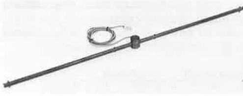
Figure 11. Reinforcement acoustic gauge.
