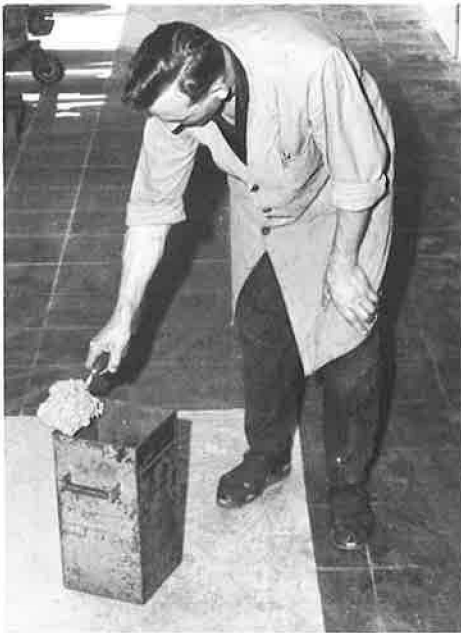
Figure 3. Filling of the container by slowly dumping concrete from trowel over borders of container.
