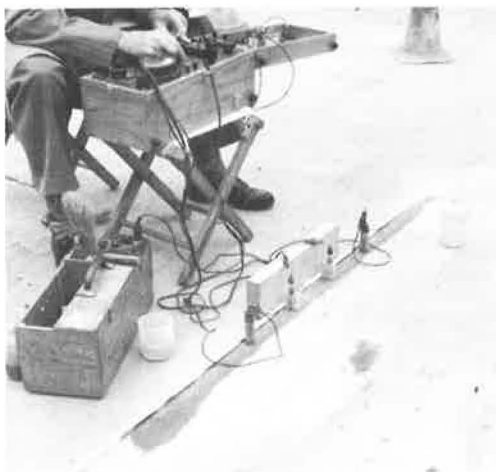
Figure A-3. Typical miniature resistivity test in progress on concrete pavement.
