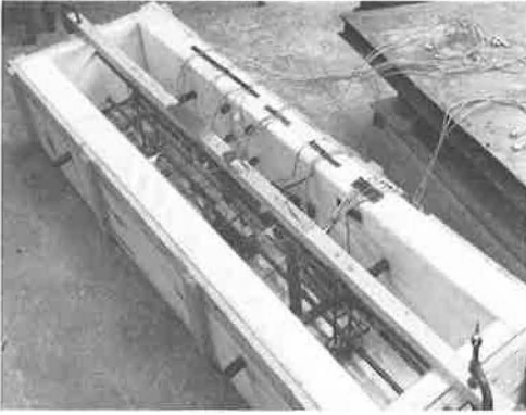
Figure 9. Mold for simulated-deck experiment, River Aire Bridge.
