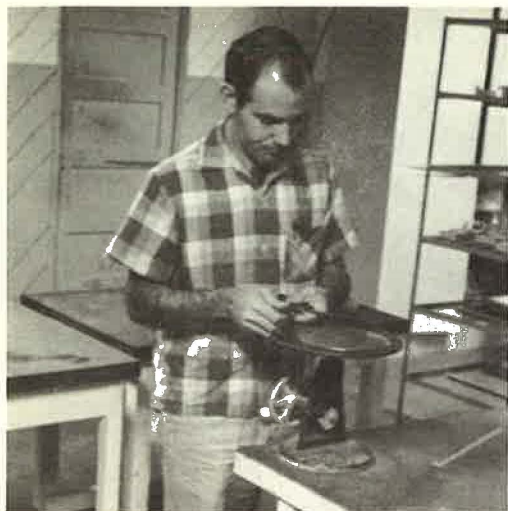
Figure 1. Determining flow of the hydraulic cement mortar.
