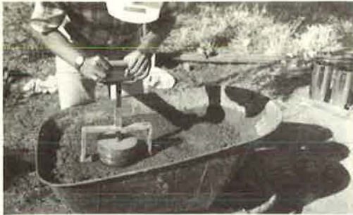
Figure 15. Measuring concrete slump with a Kelly ball.
