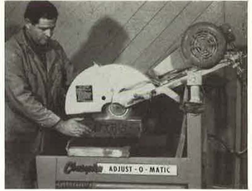
Figure 4. Sawing mortar specimen to expose surface for microscopic examination.
