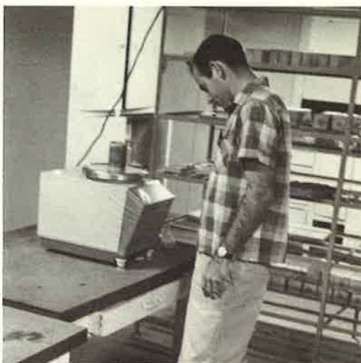
Figure 2. Determining air content of the hydraulic cement mortar.
