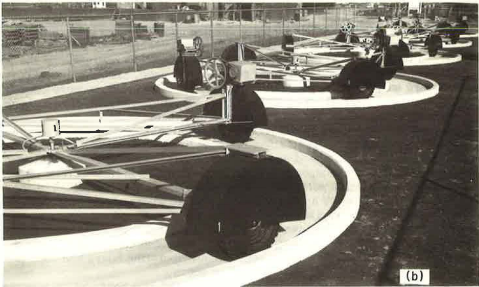
Figure 9. The traffic simulators (test rigs) showing (a) drive mechanism and (b) wheelpaths.
