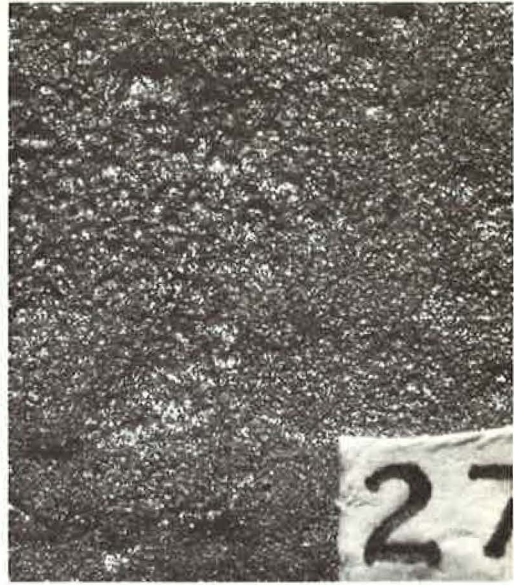
Figure 38. Example of deep pitting beneath protective lacquer—coupon exposed for 12 months on a test vehicle.
