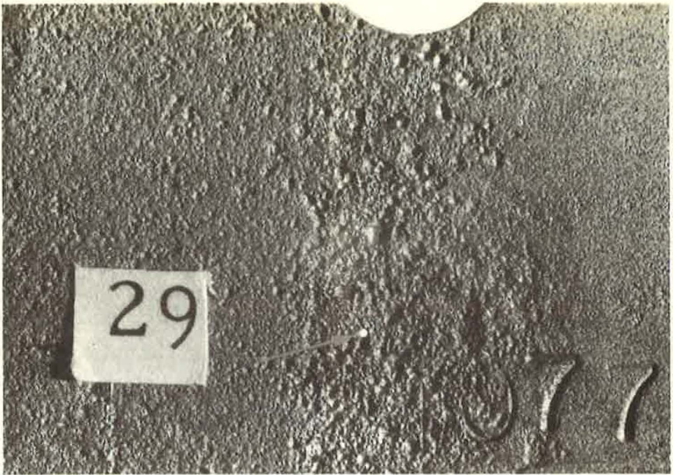
Figure 39. Example of deeply pitted area beneath protective lacquer, showing actual perforation—coupon exposed for 19 months in Test Rig No. 5.
