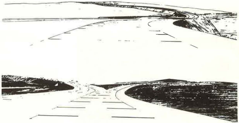
Figure 8. The same after correction by offsetting the alignment: both arms can be seen at 500 yd (top), and the division itself is clearly visible at 300 yds (bottom).
