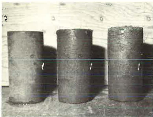
Figure 10. Champaign County till after 0, 3, and 12 freeze-thaw cycles (96-hr curing).
