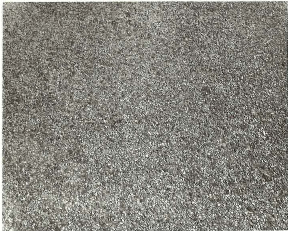
Figure 1. RC-4 with no-strip additive, Aug. 10, 1965.
