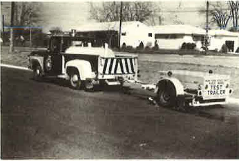
Figure 1. Skid trailer and tow truck.
