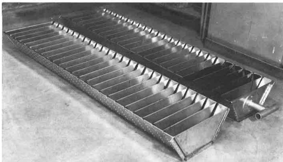
Figure 2. Calibration trough, disassembled.
