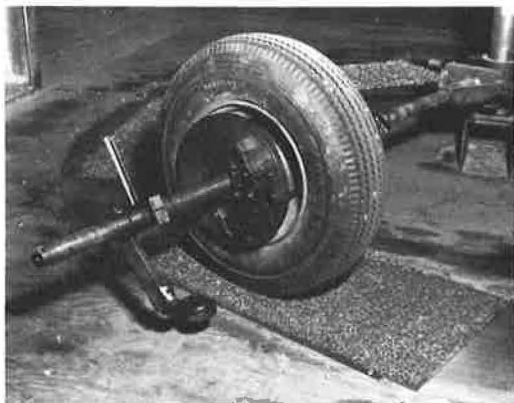
Figure 5. Laboratory polishing machine.
