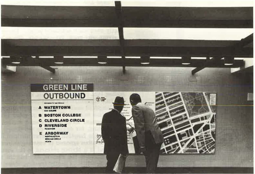
Figure 3. Typical map units at a mezzanine, including diagrammatic map of rapid-transit lines, letter coding for branches of a line, and a neighborhood map.
