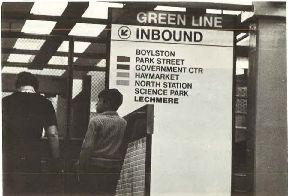
Figure 4. Typical sign at a decision point (top of stair) giving line name, platform direction (inbound), sequence of stops and identifying transfer stations to other lines (color bars).
