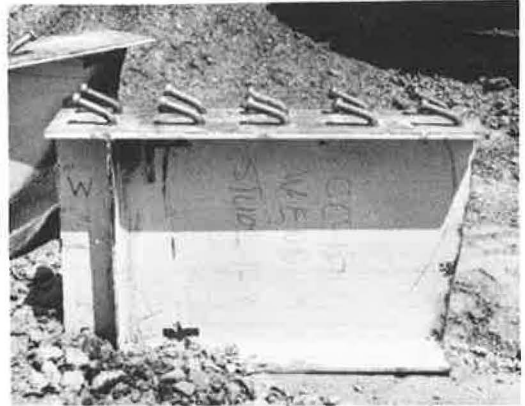
Figure 13. Studs at the end of beam CC-1F after fatigue testing.
