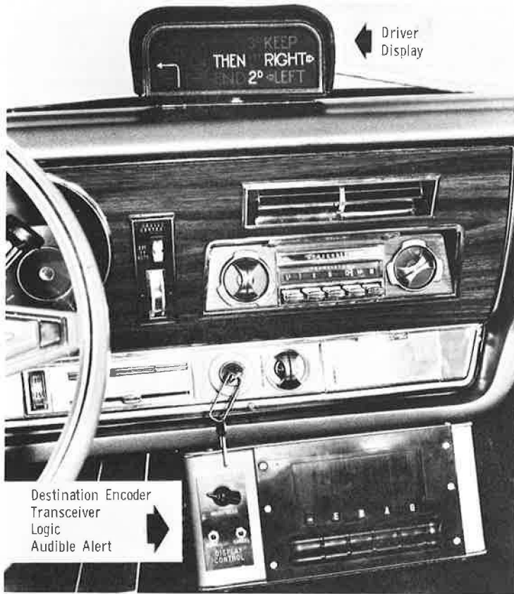
Figure 1. Vehicle Equipment—the communication antenna (not shown) is located under the rear of the vehicle.
